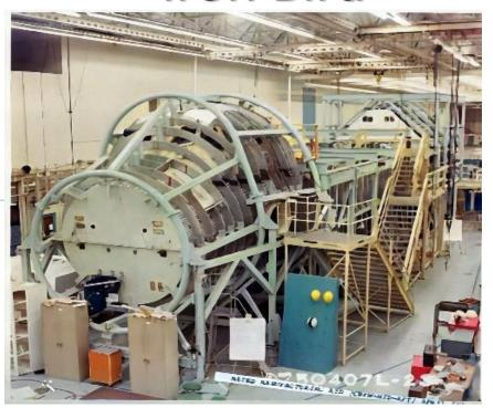
An **iron bird** is a ground-based test device used for prototyping and integrating aircraft systems during the <u>development of new aircraft designs</u>. Aircraft systems are installed into the iron bird so their functions can be tested both individually and in correlation with other systems.
